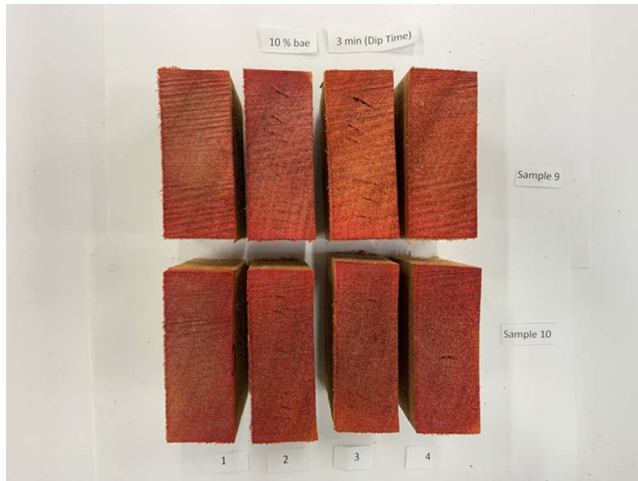
Figure 2.—Example of crosscuts from Queensland maple samples dipped for 3 minutes in a 10 percent boric acid equivalent disodium octaborate tetrahydrate solution and stored for 1 to 8 weeks (1 = 1 wk, 2 = 2 wk, 3 = 4 wk, and 4 = 8 wk) under nondrying conditions. Samples were dried and a fresh cut was made; the surface was then sprayed with a curcumin/salicylic acid indicator to develop the reddish color indicative of boron.
