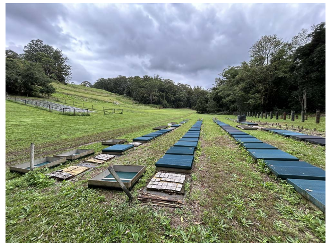
Figure 1.—Field trial set up at Nambour, Queensland showing arrangement of ground proximity arrays. Treated samples lie on concrete blocks that are enclosed and shaded by a 70 percent ultraviolet-resistant water-permeable shade cloth to create a wind-sheltered, high-humidity microenvironment to increase the risk of decay. Samples are assessed annually.
