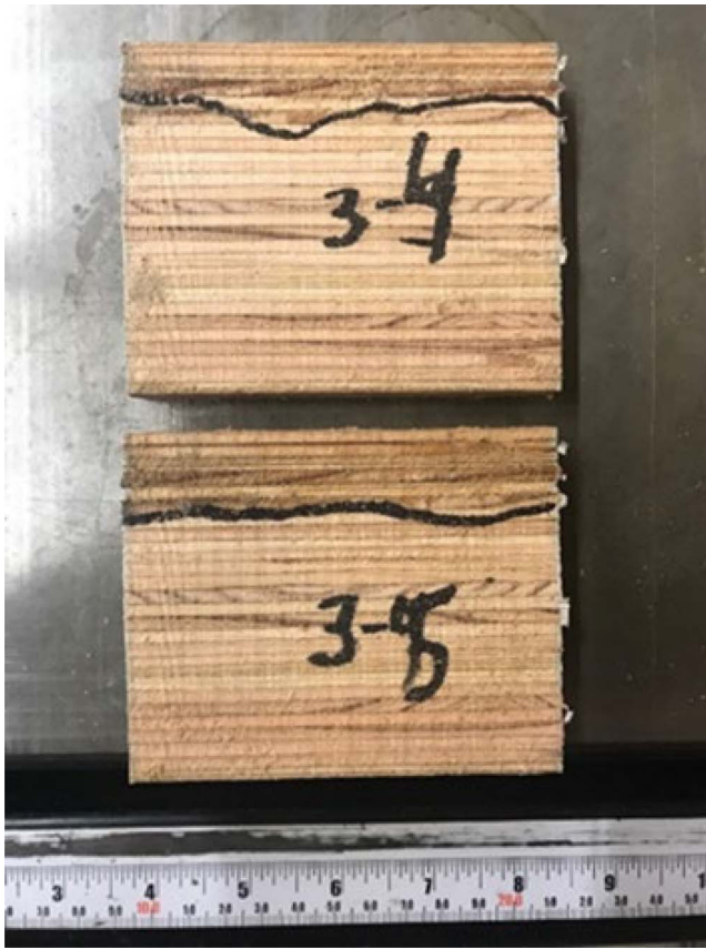
Figure 6.—Cross cuts of an mass ply panel without a water repellent showing moisture intrusion (darkened area above the marker) after 7 days of wetting.
