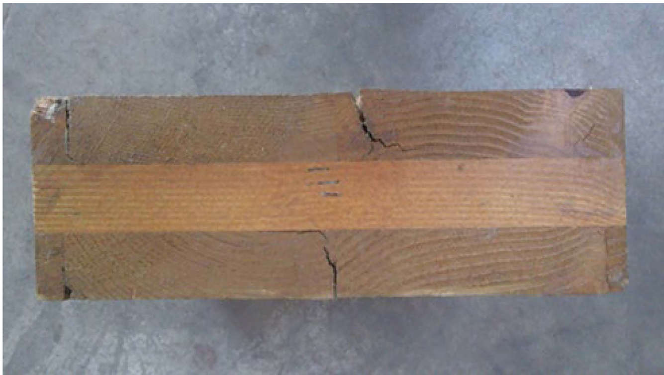
Figure 2.—Example of a Douglas fir cross-laminated timber panel section exposed to natural rainfall for 30 days and air dried for 2 years showing checking and delamination.
