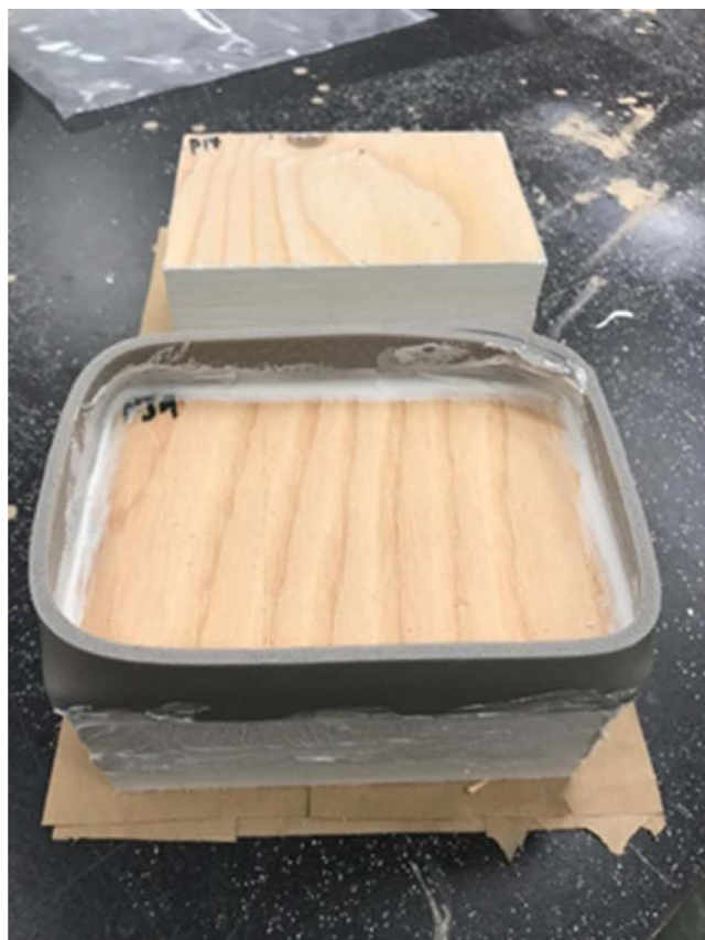
Figure 3.—Examples of a mass ply panel block: before sealing (top); sealed with the water well (bottom).
