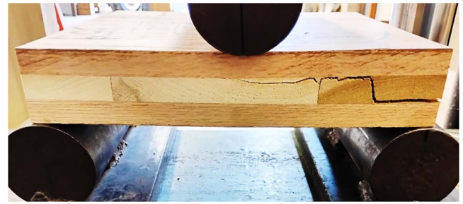
Figure 3.—Shear strength test setup of the red oak hybrid (ROYP) CLT specimen during testing.
