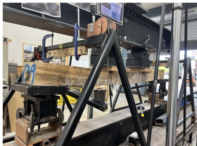
Figure 2.—Demonstration of static bending test.
