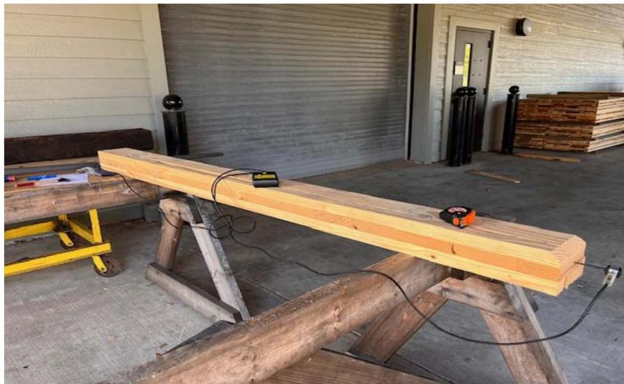
Figure 2.—Nondestructive evaluation setup using Fakopp microsecond timer.
