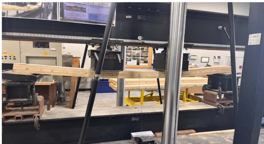
Figure 3.—Static bending setup using Instron 600 KN universal testing machine.
