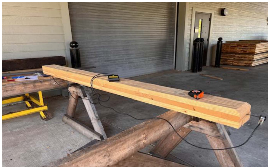
Figure 2.—Nondestructive evaluation setup using Fakopp microsecond timer.
