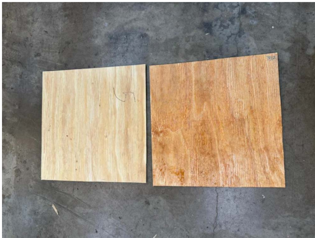
Figure 1.—An even distribution of phenol–formaldehyde resin on softwood veneer.
