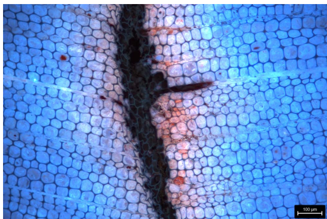
Figure 1.—A phenol formaldehyde bond line between southern yellow pine veneers imaged using an ultraviolet filter cube. Image shows the color differences between wood and the adhesive under the filter.
