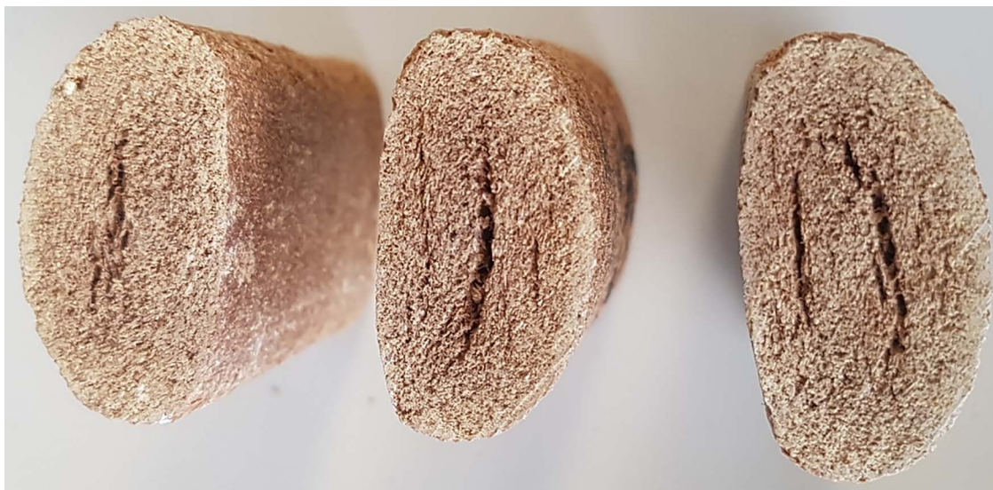
Figure 6.—Internal cracks and voids formed following microwave-induced curing of extrusion-printed wood–sodium silicate samples.
