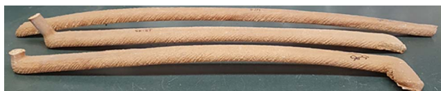
Figure 2.—Geometric distortions induced from rapid cooling of extrusion-printed wood–sodium silicate samples.
