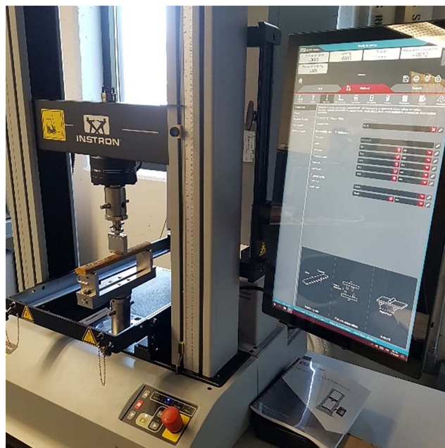
Figure 3.—Three-point flexure test setup.
