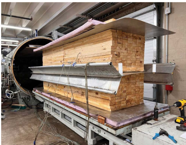
Figure 1.—Stringer load with three-plate, middle-wing electrode system with installed fiber-optic temperature probes ready to be loaded into the radio frequency-chamber.
