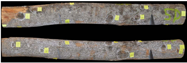
Figure 6.—Top and side photos of Log 10 showing crook and sweep.
