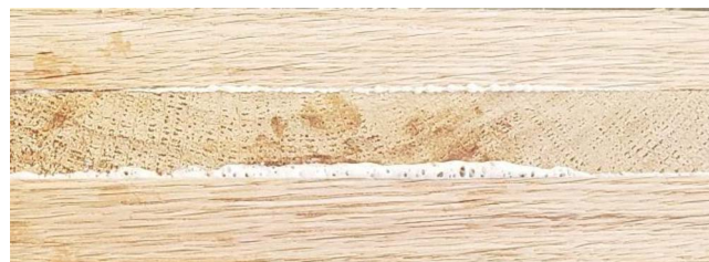
Figure 1.—The appropriate level of squeeze-out along the bond lines after pressing.
