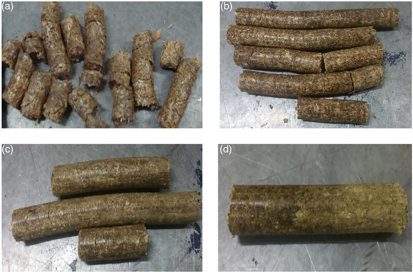
Figure 2.—Four different surface-quality categories of biomass moulding fuel (BMF) briquettes.
