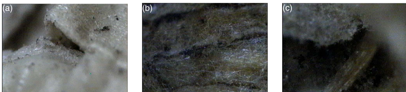
Figure 6.—Microstructure of briquettes under different moisture content.
