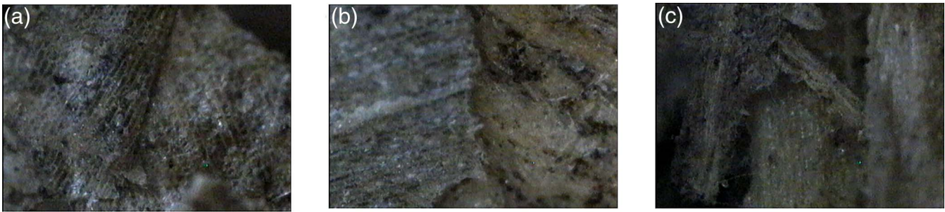
Figure 5.—Microstructure of briquettes under different length–diameter ratios.
