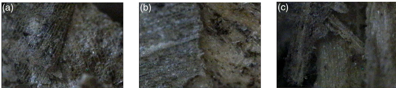
Figure 5.—Microstructure of briquettes under different length–diameter ratios.
