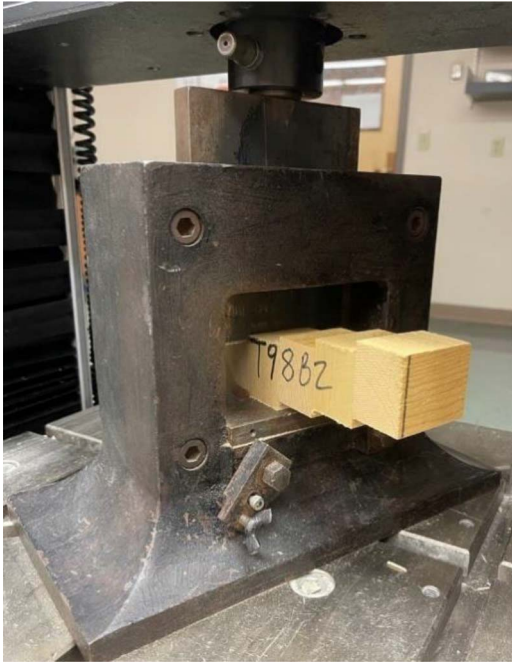
Figure 4.—Block shear test setup.
