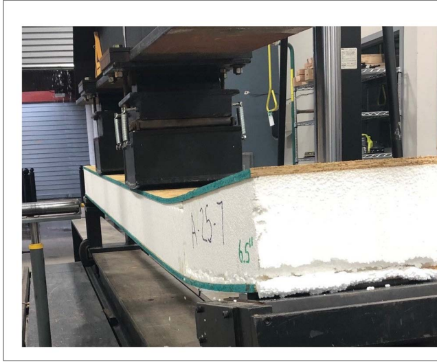
Figure 3.—Failure in 6.5-in-deep structural insulated panel. Failure initiated at a butt-jointed foam discontinuity in all specimens.
