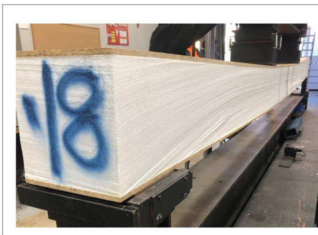
Figure 1.—Full-scale 12.25-in-deep specimen in the one-third-point testing fixture. Note string deflection gauge affixed at the neutral axis at mid-span to capture maximum deflection.
