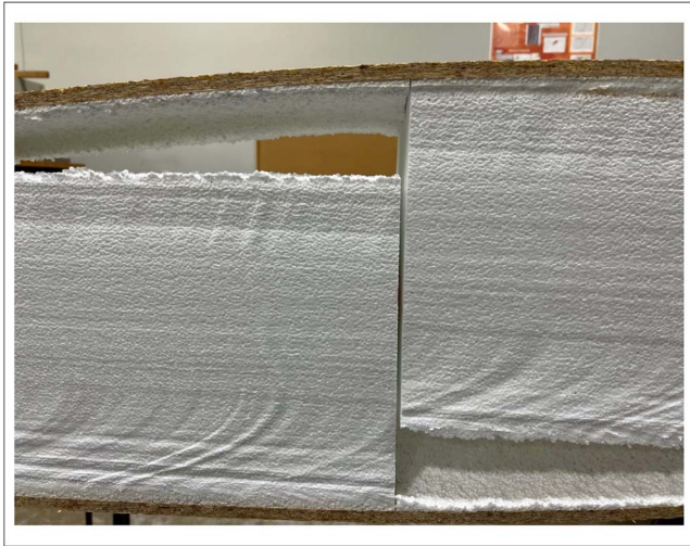
Figure 5.—Shear failure mode in exemplar 31.1-cm (12.25-in.)-class beam. All beams in this depth class failed by this same mode.
