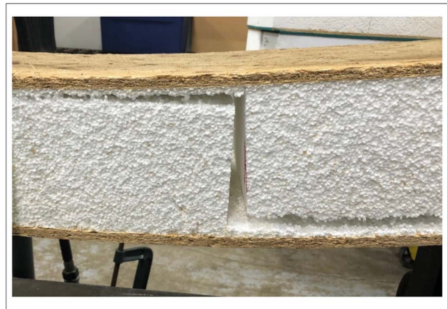
Figure 4.—Shear failure mode in exemplar 16.5-cm (6.5-in.)-class beam. All beams in this depth class failed by this same mode.
