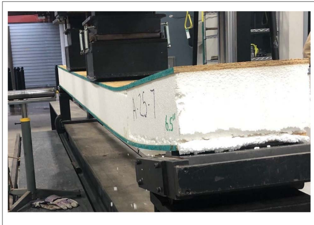
Figure 3.—Photograph of 16.5-cm (6.5-in.)-class beam in the testing machine at the time of failure.
