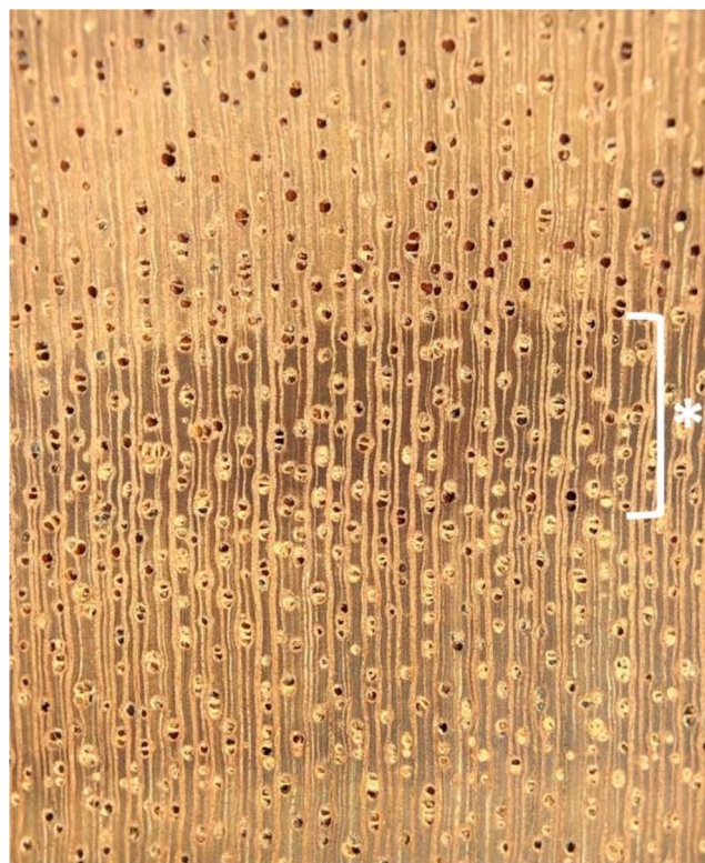
Figure 2.—Macroscopic image of Khaya sp. Growth rings delineated by a darker zone of fibrous tissue (*). Note the vessel porosity (diffuse-porous), arrangement (radial pattern), and grouping (multiples of two to three). Rays of distinct widths.
