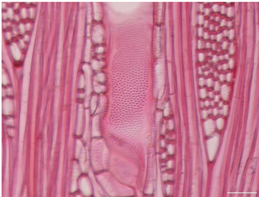
Figure 5.—Tangential section of Khaya sp. Intervessel pits minute, round, or irregularly polygonal. Fibers thin- to thick-walled, usually septate. (Scale bar 50 \mu m).
