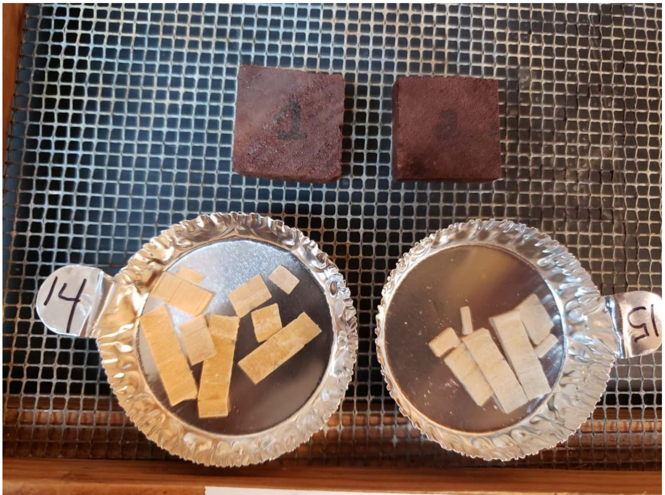
Figure 10.—African mahogany (top) and southern yellow pine control samples (bottom) after exposure to subterranean termites.
