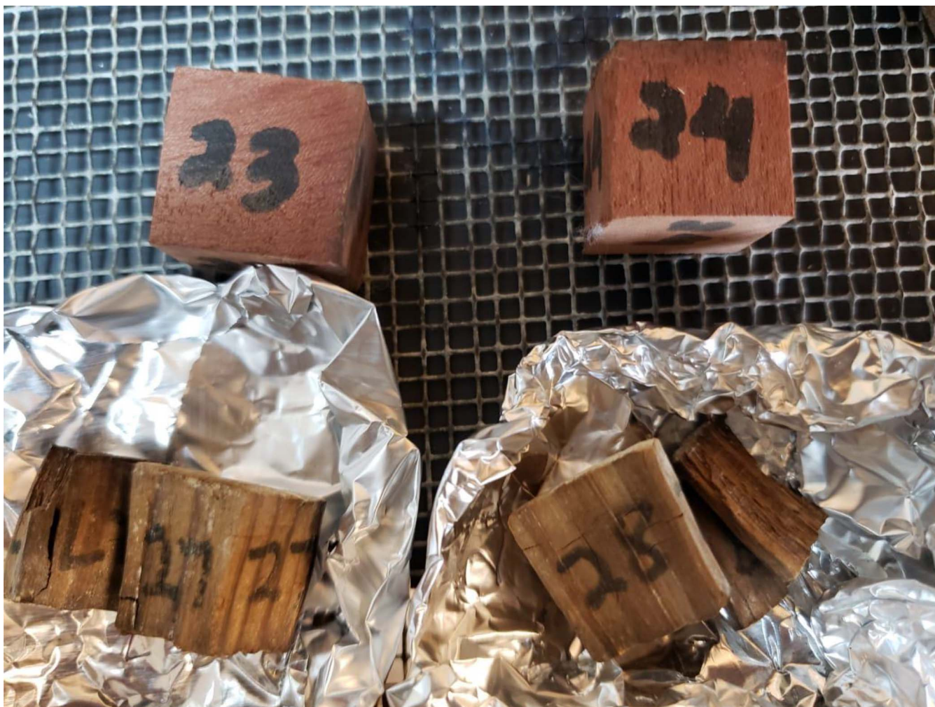
Figure 11.—African mahogany (top) and southern yellow pine control samples (bottom) after exposure to the brown-rot fungus, Gloeophyllum trabeum .
