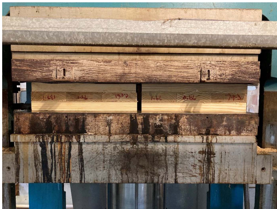
Figure 2.—3-ply cross-laminated timber (CLT) panels in Dieffenbacher laboratory hydraulic press.
