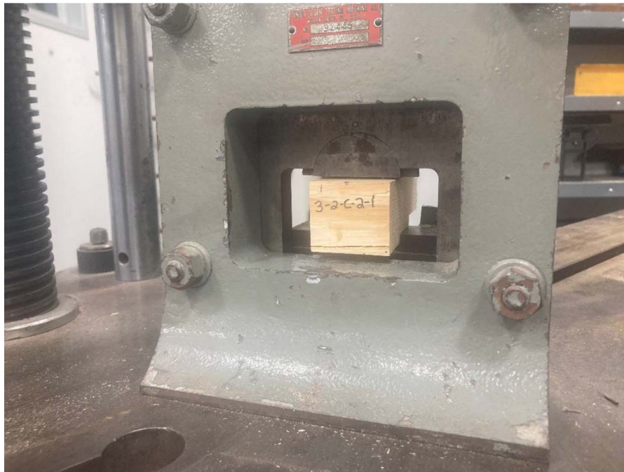
Figure 6.—Block shear specimen in block shear test setup.
