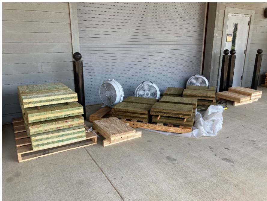
Figure 3.—Cross-laminated timber (CLT) panels under breezeway air-drying.
