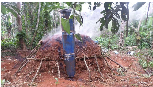
Figure 2.—Production of pyrolygneous acid by a Casamance millstone.
