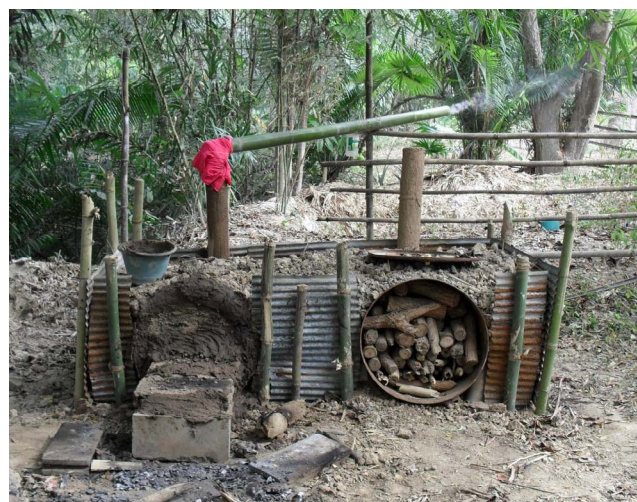
Figure 1.—Pyrolytic acid production process by 200-liter drum furnaces.
