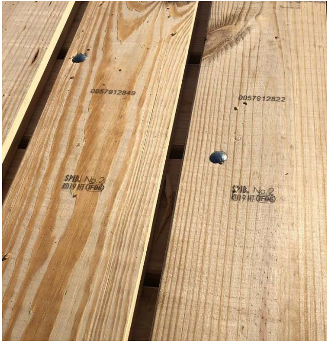
Figure 2.—Examples of grade stamps that were visible on one of the surfaces of one of the parent mats.
