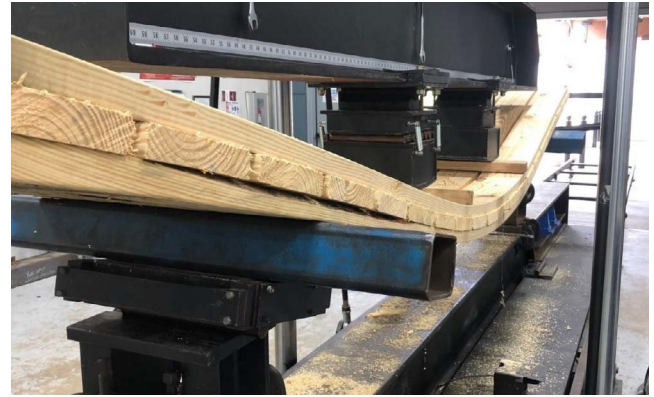
Figure 3.—One of the test specimens in the universal testing machine while being destructively evaluated in 1/3-point bending.
