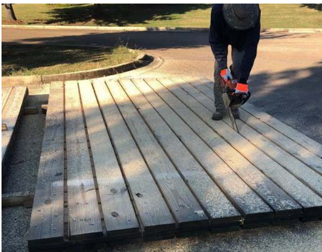
Figure 1.—Chainsaw ripping of each 243.84 by 426.72-cm (8 by 14-ft) parent mat into four test specimens, each approximately 60.96 cm (2 ft) wide.
