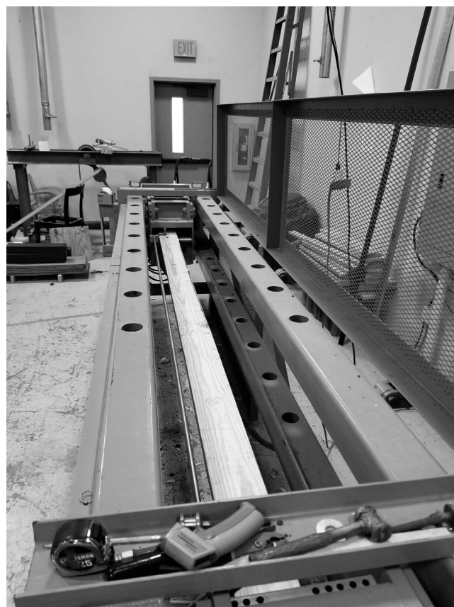
Figure 2.—The test setup used to determine tension parallel to the grain properties.
