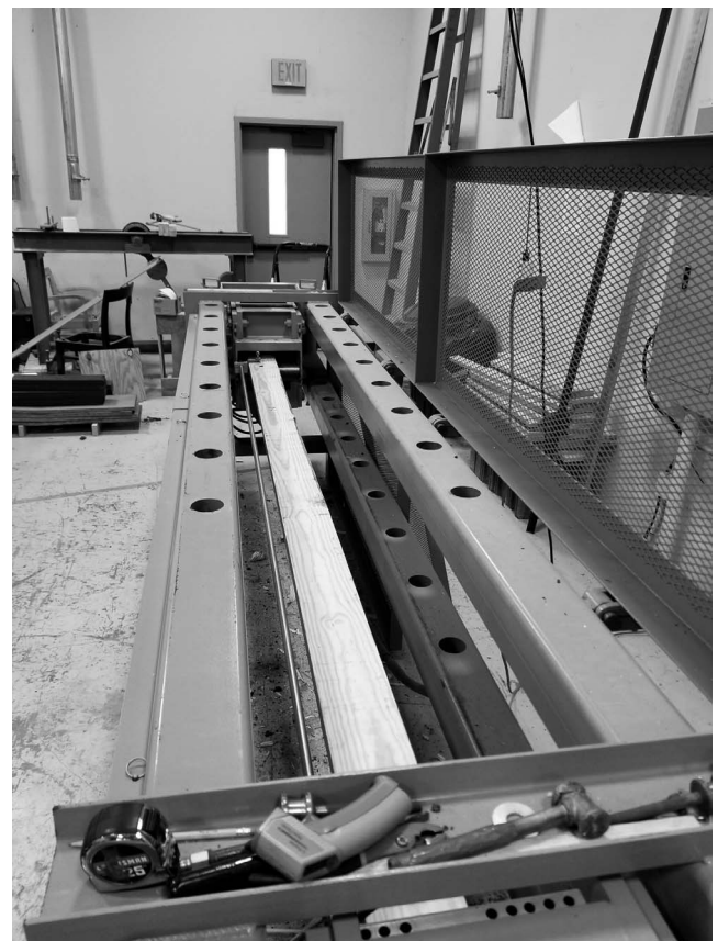
Figure 2.—The test setup used to determine tension parallel to the grain properties.
