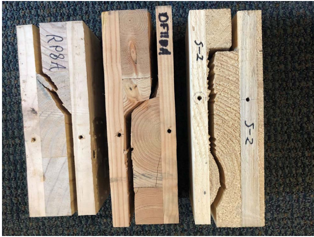
Figure 5.—Typical failure patterns in rolling shear test. From left, radiata pine, Douglas-fir, and spruce. Each of these samples was treated but the controls did not look different in terms of failure pattern. The holes are where the linear variable differential transformers (LVDT) brackets were located.
