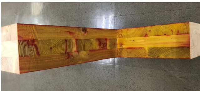
Figure 6.—CLT panel that was treated in a vacuum bag. A corner section was cut and removed from the panel after treatment and the interior sprayed with boron indicator. Red color indicates the presence of boron.
