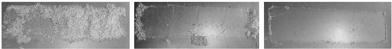
Figure 4.—Images of platens coated (left to right) with polymeric diphenylmethane diisocyanate (pMDI) containing 0, 10, and 20 percent soy flour (left to right).
