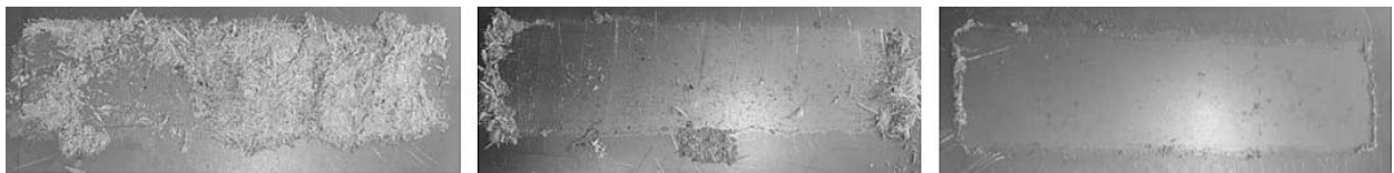
Figure 4.—Images of platens coated (left to right) with polymeric diphenylmethane diisocyanate (pMDI) containing 0, 10, and 20 percent soy flour (left to right).
