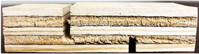
Figure 1.—Kerfed sample for lap shear.
