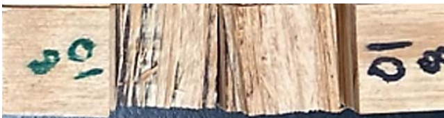
Figure 3.—Lap shear sample.
