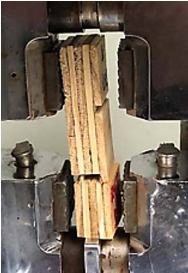
Figure 2.—Testing lap shear sample.
