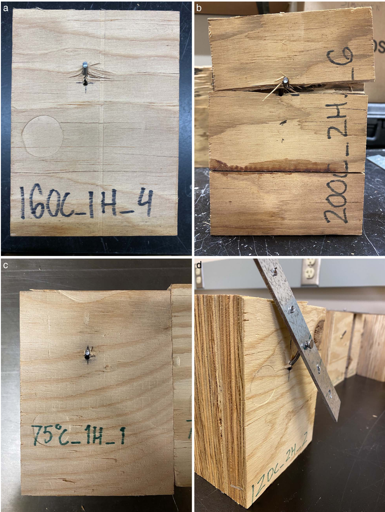
Figure 5.—Failure modes of nail connection specimens: (a) combination of nail pullout, broken nailhead, and wood damage; (b) wood crushing and splitting; (c) broken nailhead without wood damage; and (d) nail pullout and wood crushing.
