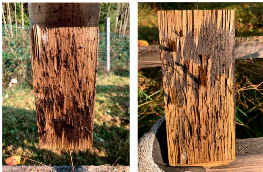
Figure 4.—An example of delamination failure in one of the gamma joint test units. The lighter colored sections indicate wood failure.
