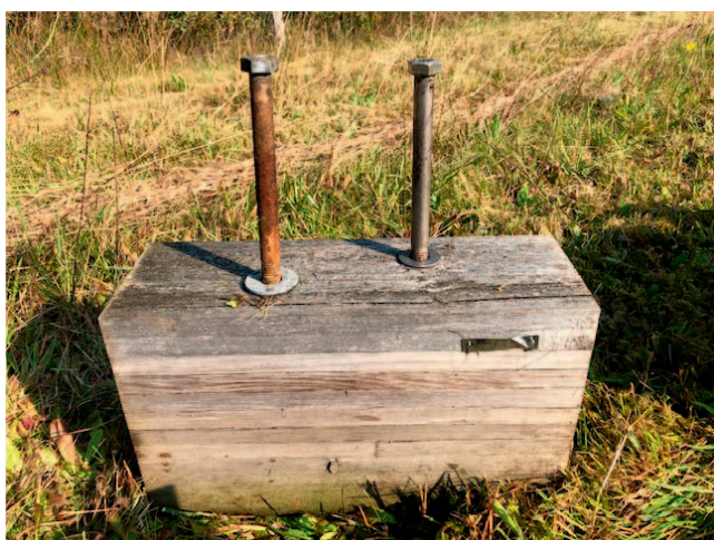
Figure 2.—Ground proximity test unit showing galvanized (left) and stainless-steel (right) bolts after 10 years of exposure in Maple Ridge, British Columbia.
