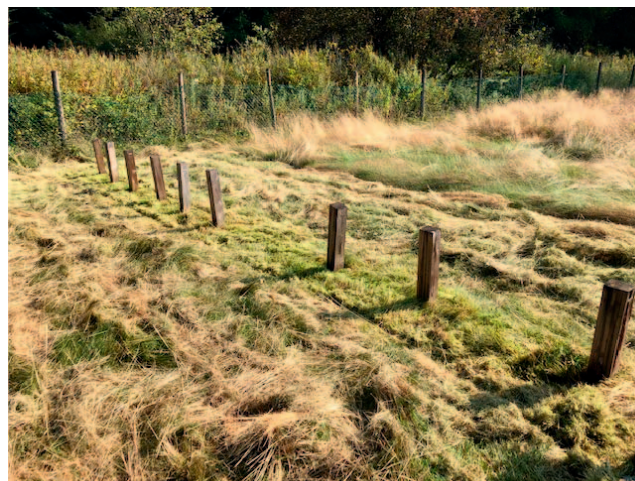
Figure 3.—Treated 5-ply glulam samples from one quadrant in the ground contact test after 10 years of exposure in Maple Ridge, British Columbia.
