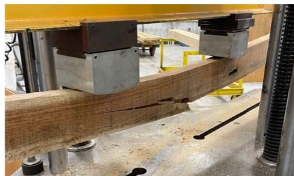
Figure 2.—Red oak lumber on Tinius Olsen machine before (upper panel) and after failure (lower panel) with the type of failure in static bending cross-grain tension (ASTM D143-14 [ASTM 2017a]).
