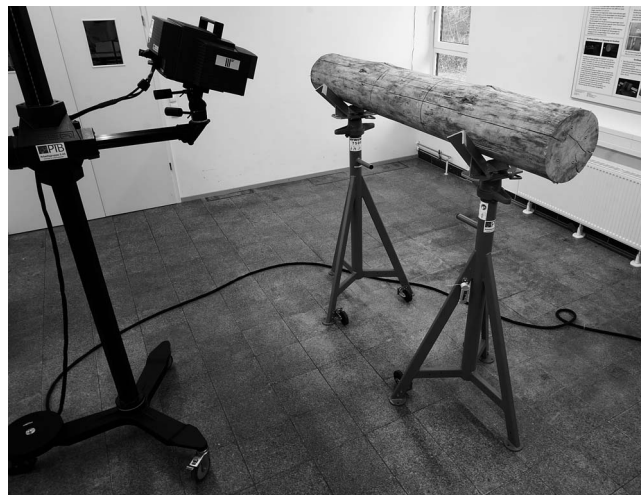
Figure 1.—Log (length 2 m, diameter 280 mm) on two supports in Bessel configuration before the start of fringe projection scanning. The scanning head of the fringe projection system containing the pattern projector and the cameras is seen on the left.
