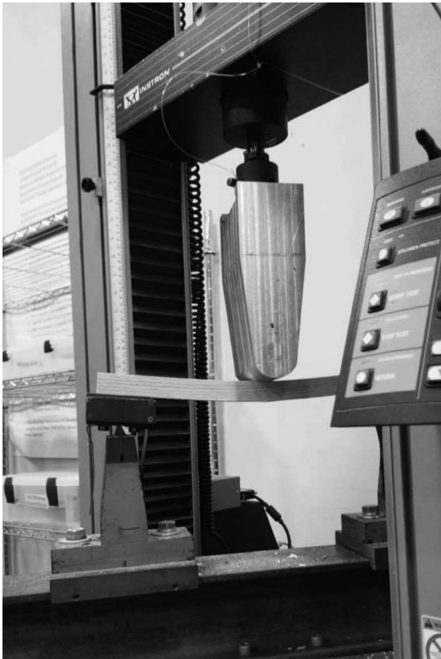
Figure 2.—Center point bending test setup (Sample 3).
