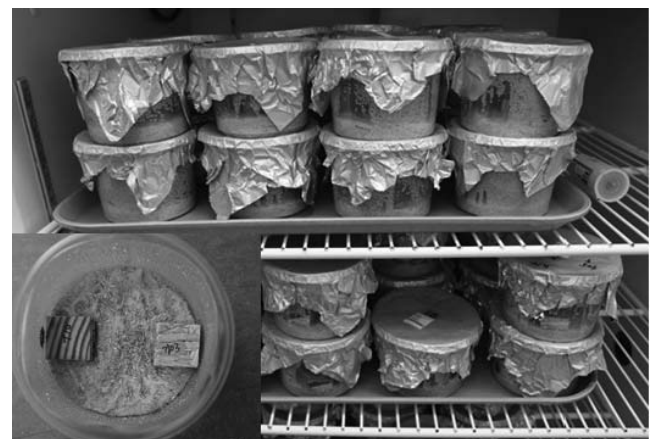
Figure 1.—Termite containers in the environmental chamber. The inset (lower left) shows the arrangement of the samples in one container and how termites were initially congregated in the center after being added.
