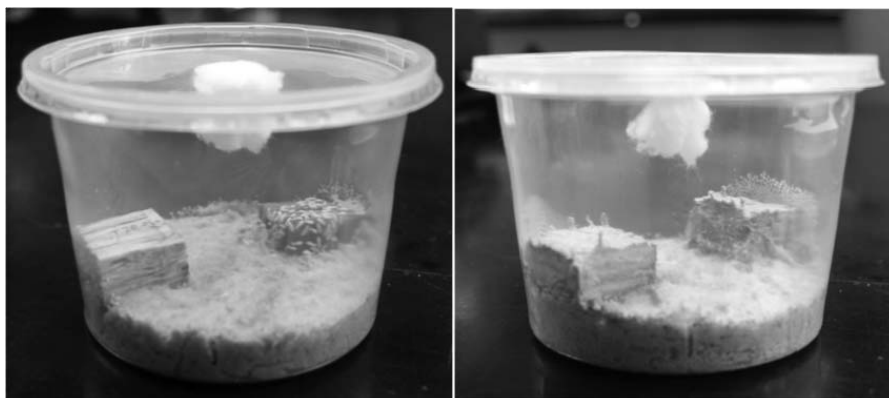
Figure 4.—Three-week photos showing termite preference for SYP in SYP versus OSB20 choice test (left) and no obvious preference in the OSB choice test, OSB0 versus OSB10 (right, samples also encased in moist sand).
