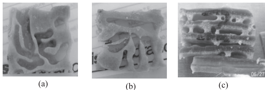
Figure 4.— C. formosanus damage on spruce blocks (a and b) after choice testing against southern yellow pine (c).
