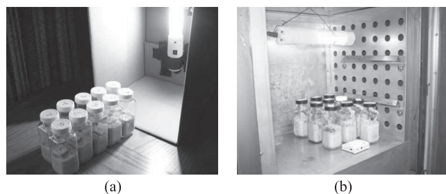
Figure 2.—Layout for 100 percent light photoperiod for (a) Reticulitermes flavipes and (b) Coptotermes formosanus .
