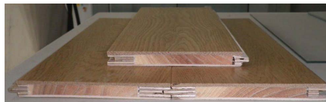
Figure 1.—The construction of Metasequoia -based three-layer parquet flooring.
