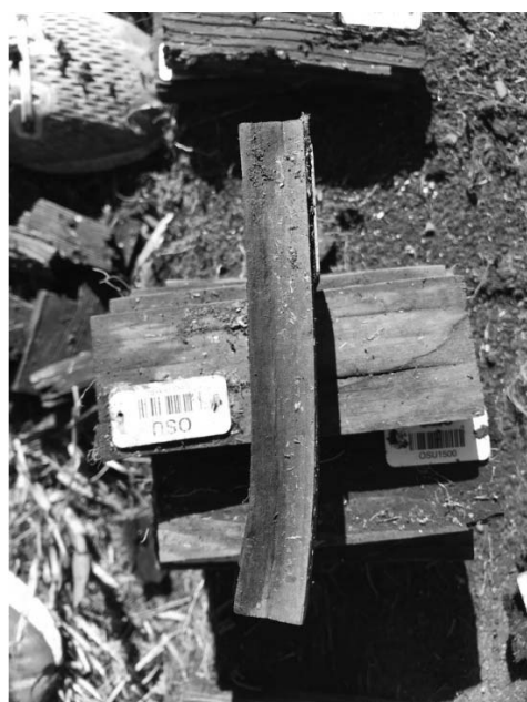
Figure 1.—Example of a thermally modified sample of Douglas-fir showing extensive curvature after 57 months of exposure in a ground proximity test in Hilo, Hawaii.
