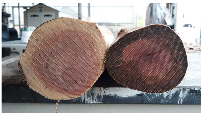
Figure 2.—Healthy (left) and C. lukuohia -infested (right) wood from DOT penetration assays. The dark staining on the diseased bolt is associated with C. lukuohia colonization.
