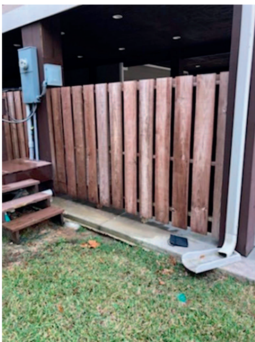
Figure 5.—No checking on chromated copper arsenate/oil-treated fence boards on the exposed (left) or protected (right) side after more than 8 years of exposure.
