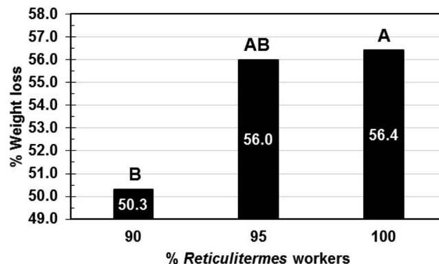
Figure 4.—Percentage of weight loss of southern pine sapwood blocks after 4 weeks exposure to varying Reticulitermes flavipes soldier:worker ratios (means with the same letter are not significantly different at P = 0.05 ).
