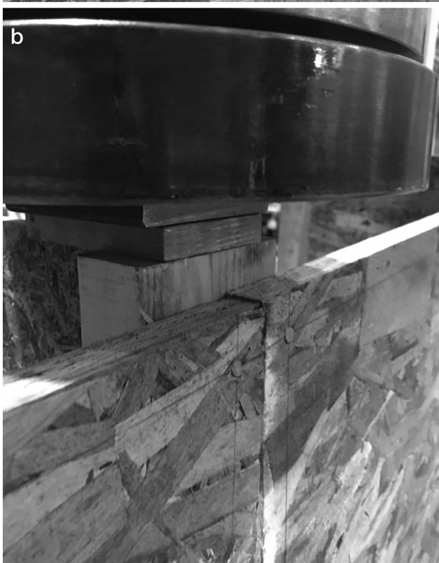
Figure 16.—The upper panel conditions after peak loads for two typical specimens: (a) conventional specimen with blocking, no. 3 and (b) panelized specimen without blockings with staggered nailing, no. 1.
