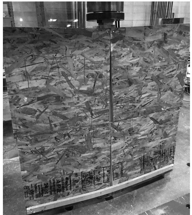
Figure 17.—Typical failure mode for panelized specimens (panelized specimen without blockings with staggered nailing, no. 1).
