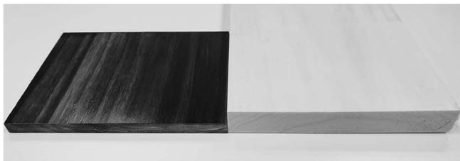
Figure 1.—Left: Thermo-hydro-mechanical and phenol-resin-treated poplar panel; right: unmodified poplar.
