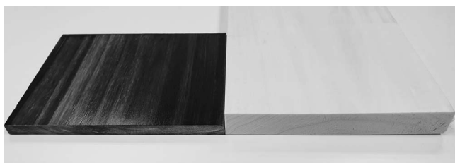
Figure 1.—Left: Thermo-hydro-mechanical and phenol-resin-treated poplar panel; right: unmodified poplar.
