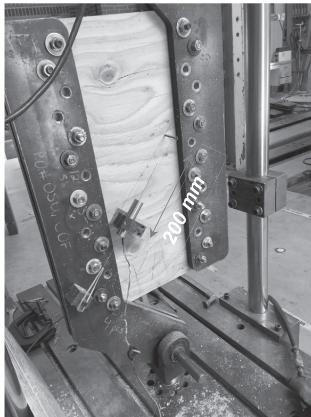
Figure 2.—Linear variable differential transformers installed on plywood.
