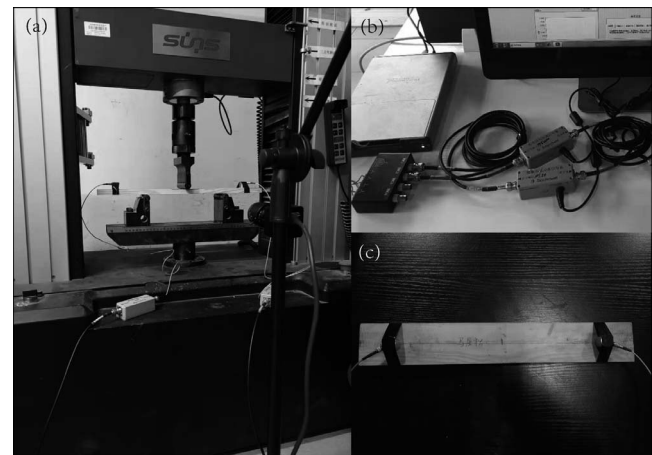
Figure 2.—Hardware composition of three-point bending test. (a) Testing setup. (b) Acoustic emission equipment. (c) Air-dried test-piece.
