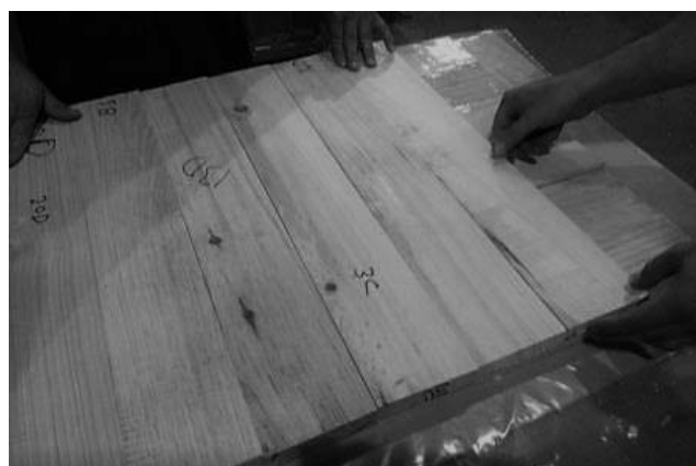
Figure 4.—Layup of the panel.
