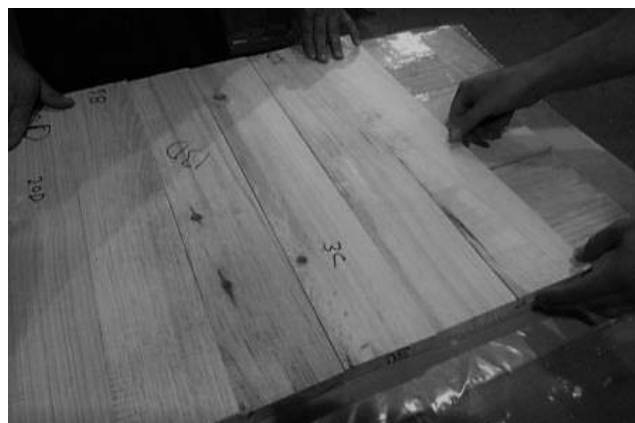
Figure 4.—Layup of the panel.
