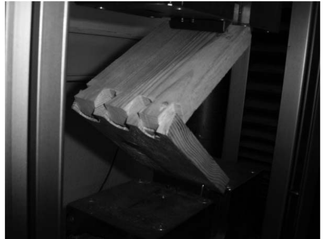
Figure 7.—Scotch pine + 84° angle + Desmodur-vinyl triketonol acetate.
