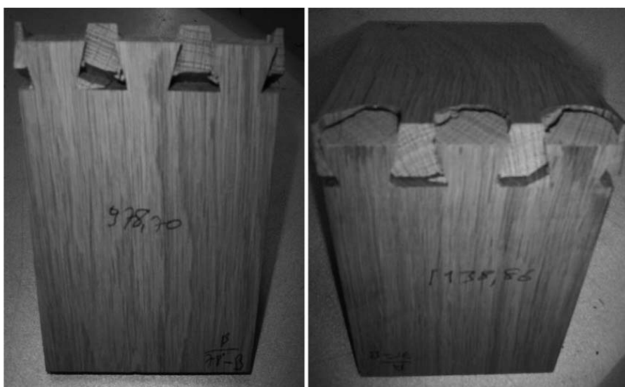
Figure 10.—Failure modes for European oak + 87° angle + polyvinyl acetate.
