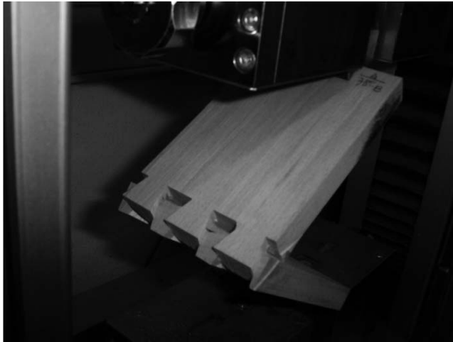
Figure 5.—Oriental beech + 81° angle + Desmodur-vinyl triketonol acetate.
