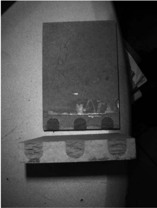
Figure 12.—Failure mode for medium-density fiberboard + 84° angle + Desmodur-vinyl trieketonol acetate.
