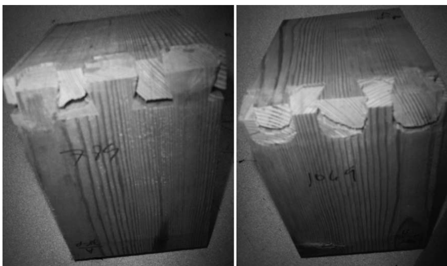
Figure 11.—Failure modes for Scotch pine + 84° angle + Desmodur-vinyl trieketonol acetate.
