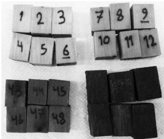
Figure 2.—Yellow-poplar control samples (upper left) and HCW-treated samples at 100°C (upper right), 140°C (lower left), and 140°C (lower right). HCW is hot-compressed water.
