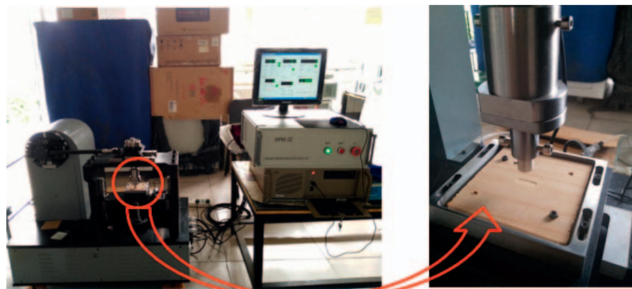
Figure 3.—Reciprocating friction and wear tester. (Color version is available online.)
