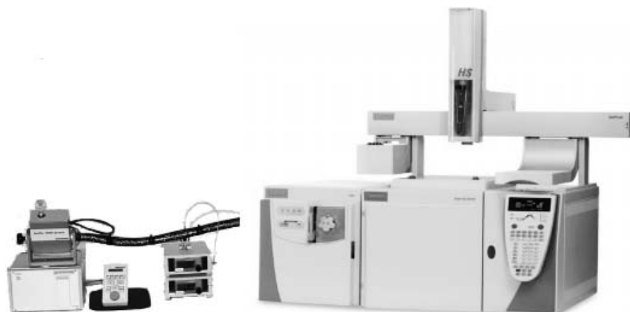
Figure 2.—Photograph of the gas chromatography coupled with mass spectrometry and olfactometry (GC-MS/O) test set-up.
