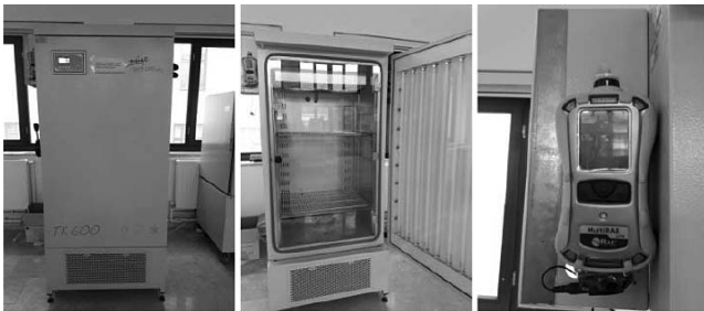
Figure 1.—Climatic test cabinet and Multi-RAE multiple gas analyzer.
