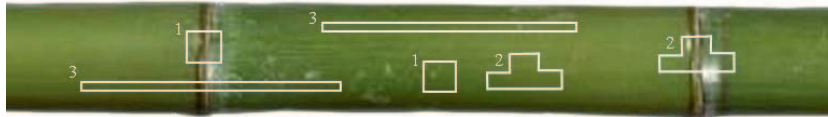
Figure 1.—Schematic diagram of specimen selection between internodes and nodes (1) compressive strength parallel to grain, (2) shear strength parallel to grain, and (3) bending test. (Color version is available online.)
