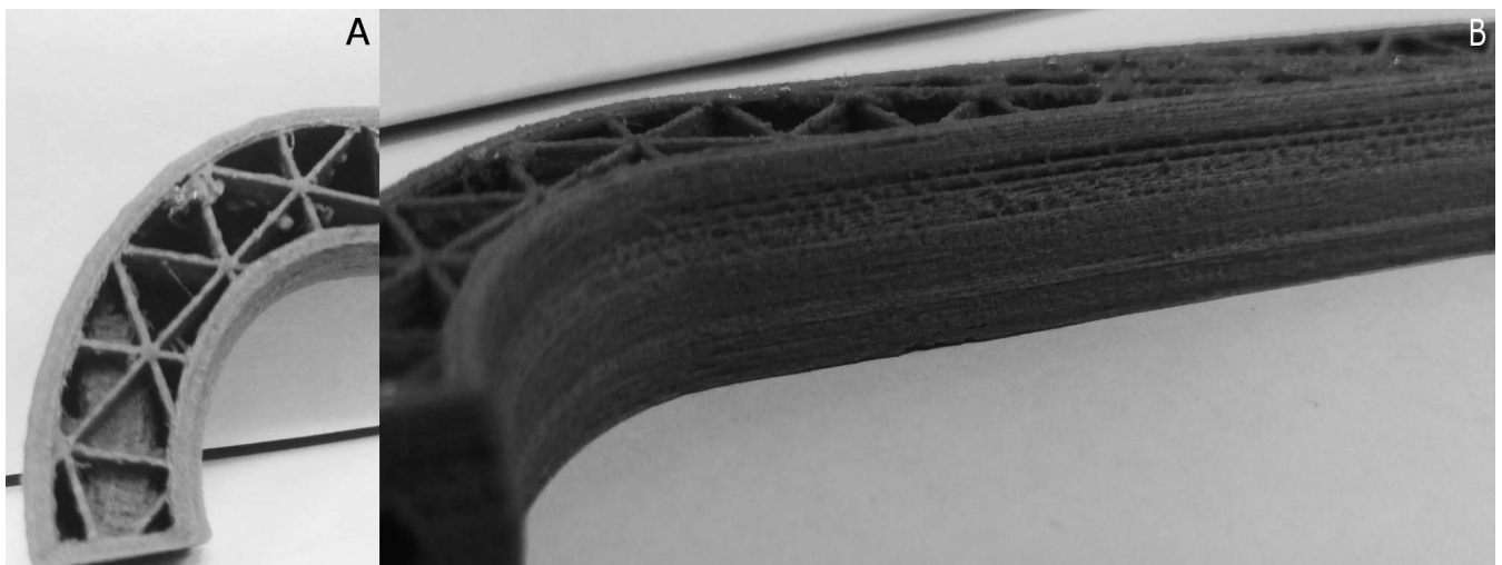
Figure 7.—(A) Internal view of a drawer handle with triangular geometry of in-fill, 30 wt% wood furniture waste, and (B) side view of same drawer handle; sidewalls have been textured during print to resemble an aesthetic wooden surface.
