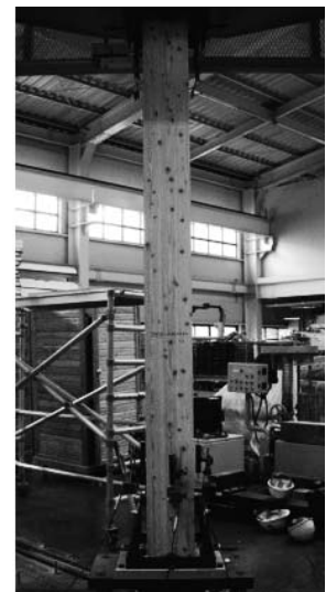
Figure 4.—Axial compression test method.
