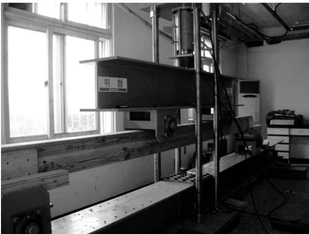
Figure 3.—Bending test method.
