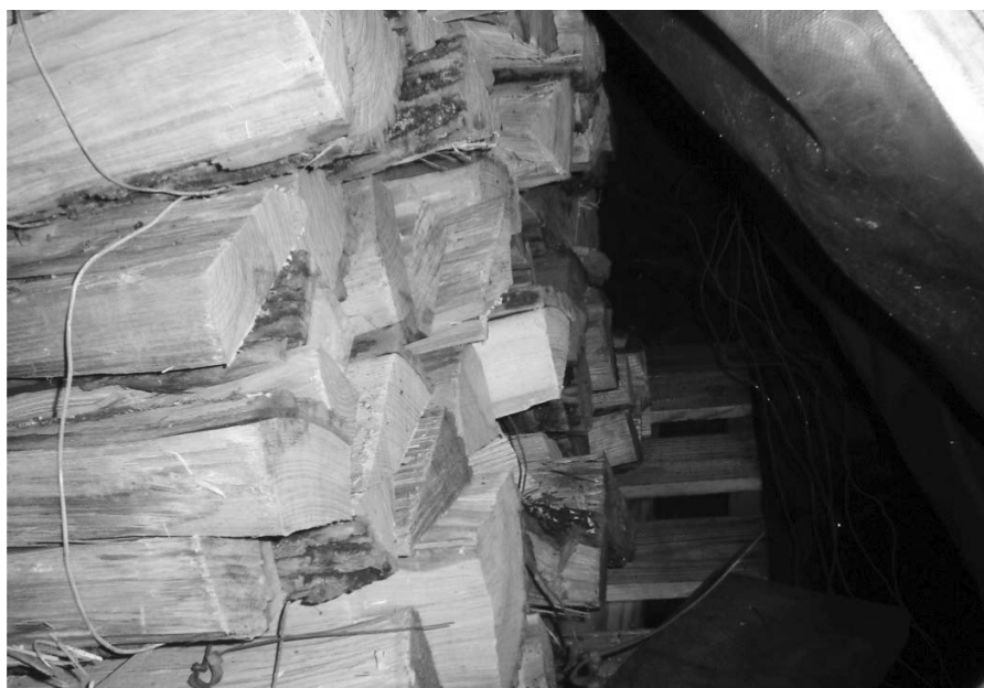
Figure 7.—Firewood bundles were loaded into the container for treatment.
