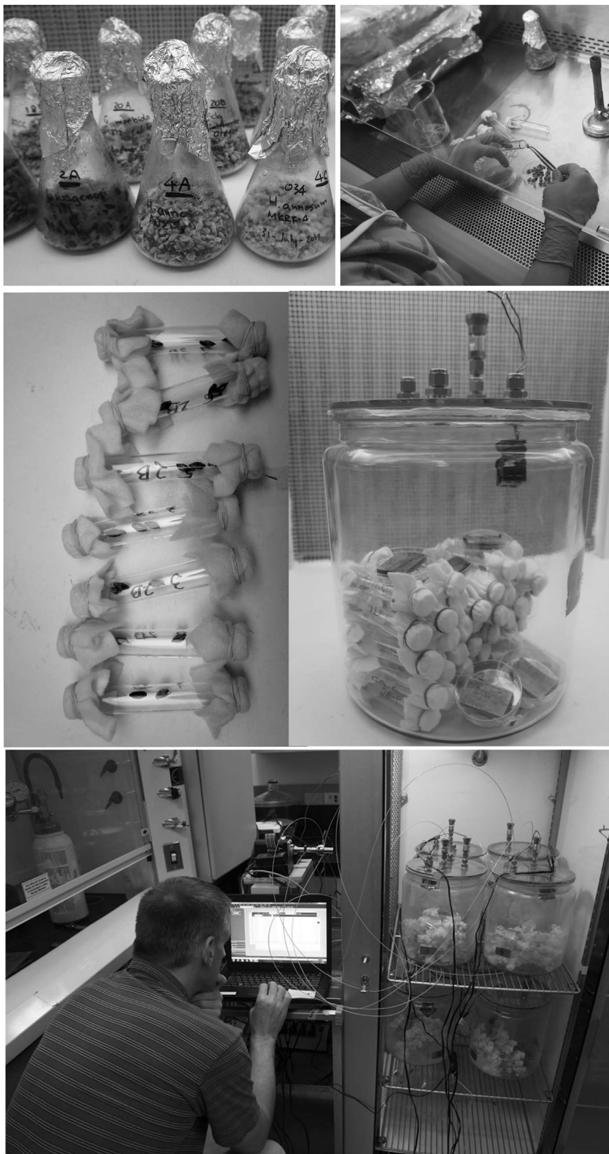
Figure 1.—Test methodology and apparatus used to simultaneously screen various fungal isolates exposed to six different gas target concentrations and a control (no fumigation). From top left to bottom right: colonized barley grains with individual fungi; distribution of grains into individual tubes; sealed tubes containing three grain pieces inoculated with a test fungus; 10-liter test jars filled with tubes containing different test isolates and petri dishes with pinewood nematode-infested wood block; and simultaneous and automatic measuring of gas concentrations in six jars using Agilent 490 micro GC.
